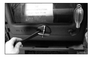
A 2mm gap at the top of the door allows additional secondary air to enter the firebox, washing over the door glass keeping it clean while also supplying necessary oxygen to the fire when the air spindle has been fully closed.
