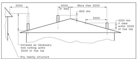
If a flue exits out of the roof within 3 meters from the ridge, the outer shield height shall be not less than 600mm above the ridge. If the flue exits further than 3 meters out from the roof ridge then it must project at least 1000mm above roof penetration. This dimension may need increased to ensure that the top of the flue is at least 3 meters away from the roof or other obstructions when measured horizontally.
